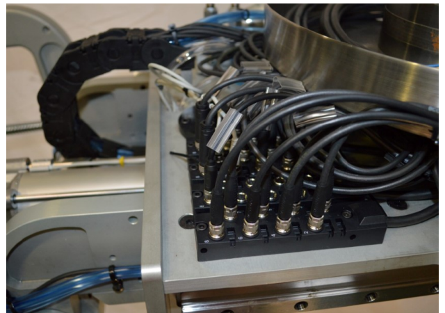
Item B- Wiring of all valves and switches to central industrial I/O block
